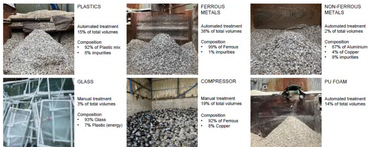
Fig. 3: Output fractions from recycling process of domestic refrigerators and freezers
